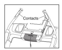
To measure your heart rate, stand on the walking platform and hold the metal contacts on the handrail for approximately ten seconds—avoid moving your hands. When your pulse is detected, your heart rate will be shown. For the most accurate heart rate reading, continue to hold the contacts for about 15 seconds.
